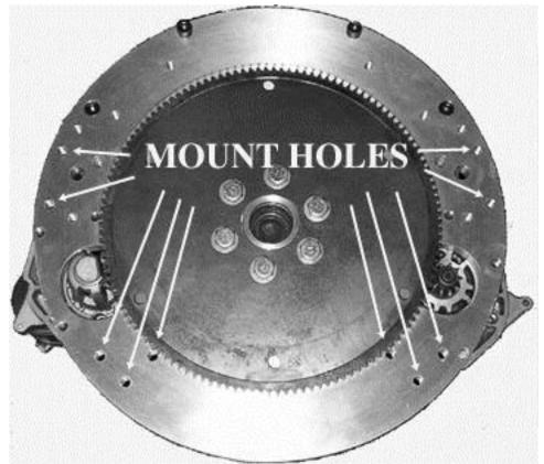
USE THE ATTACHED DRAWING TO FABRICATE THE REAR ENGINE MOUNT IF NEEDED. IF THE FRONT MOUNT, A FABRICATED MID MOUNT, AND THE REAR TRANSMISSION MOUNT ARE ALL USED ATTENTION SHOULD BE PAID TO MAKING CERTAIN THAT A "BINDING" CONDITION IS NOT CREATED. THE FRONT AND REAR MOUNTS SHOULD BEAR THE MAJORITY OF THE WEIGHT WITH THE MID MOUNT PROVIDING SIDE-TO-SIDE STABILITY.
