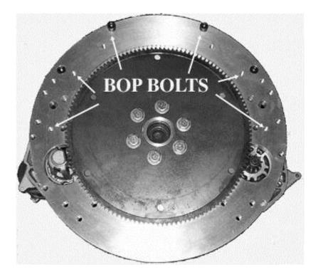
FOR CHEVROLET BOLT PATTERN TRANSMSSIONS: USE THE REMAINING TWO 1 1/2" LONG 7/16" BOLTS AT THE TOP TWO HOLES OF THE ADAPTER PLATE. USING THE TWO 7/16" SOCKET HEAD CAP SCREWS, BOLT THE PLATE TO THE BLOCK.
