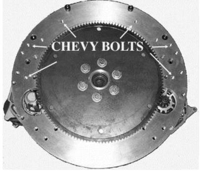
Wilcap Company P.O. Box 763 Pismo Beach, CA 93448 (805) 481-7639 www.wilcap.com Copyright 2009 All Rights Reserved. FIT UP THE STARTER MOTOR AND CHECK FOR PROPER RING GEAR TO PINION GEAR ENGAGEMENT. ADJUST IF NEEDED AND TORQUE STARTER BOLTS TO PROPER VALUE
